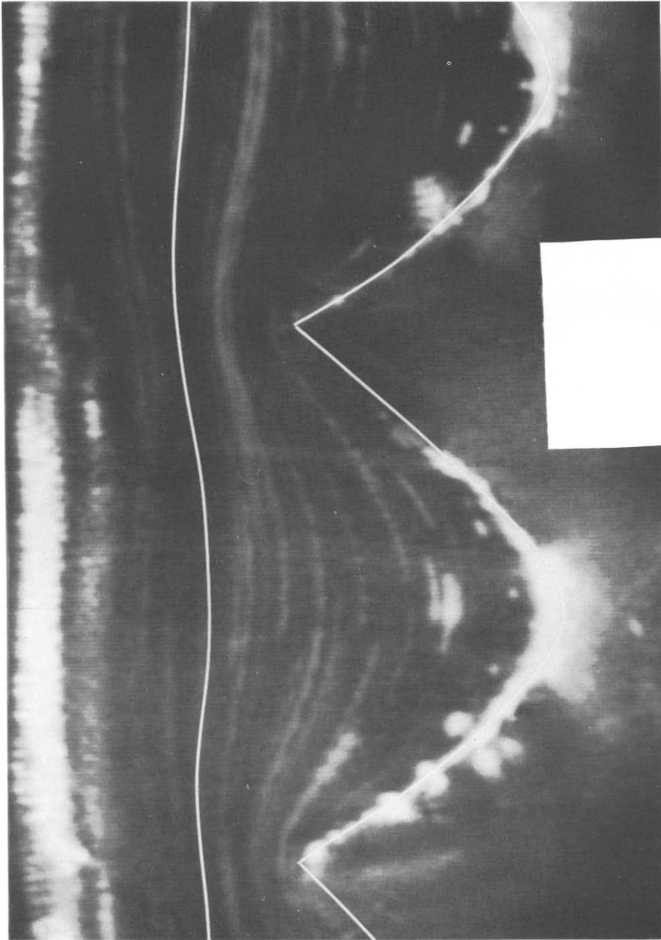
Figure 19. Streamline patterns for the flow of silicone oil on a T surface. Run 2T, h^* = 0.98 \times 10^{-3} m, Re = 0.3678 and Ca_m = 0.2122 .
